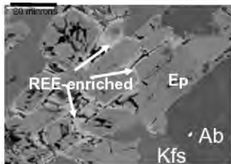
Figure 4. BSE-SEM image of epidote showing bright REE-enriched rims.
