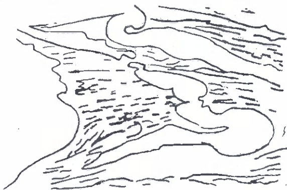
Fig. 4 Detail of Fig. 3. Note thinning to separation of the limbs and thickening in the hinge of the sandier layer.
