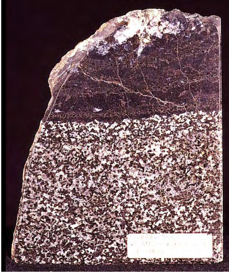
Figure 3-3: Polished slab of massive Cr-spinel layers in contact with medium-grained gabbro, Great Lakes Nickel property (Stop 3-4). White bar is 4 cm long.
