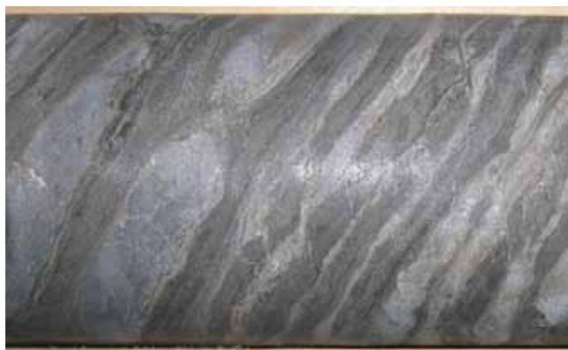
Figure 10. 4B, thick banded chert-magnetite BIF. Drill core sample 5.1cm (2") wide.
