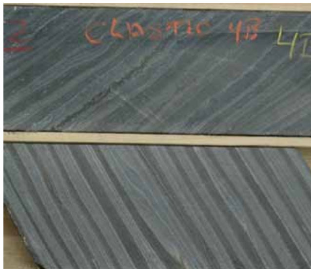
Figure 11. Laminated 4B (chert magnetite) below, clastic 4B with thin layers of green amphibole-garnet above. Drill core sample 5.1cm (2") wide.
