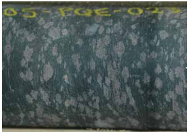
Figure 14. 4E, garnetiferous amphibolite. Drill core sample 5.1cm (2”) wide.
