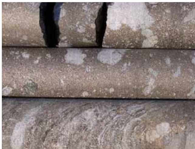
Figure 9. 4H, massive pyrrhotite exhalite with chert fragments. Drill core sample 5.1cm (2") wide.
