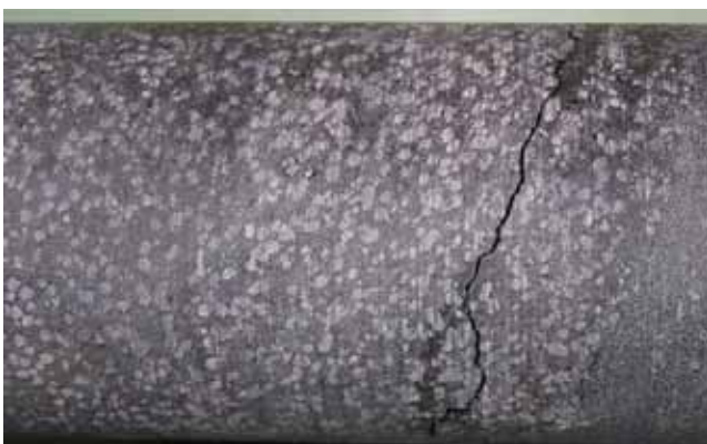
Figure 13. 4F, garnet-biotite-(Qtz-Fd)±staurolite schist; ferruginous metapelite. Drill core sample 5.1cm (2”) wide.
