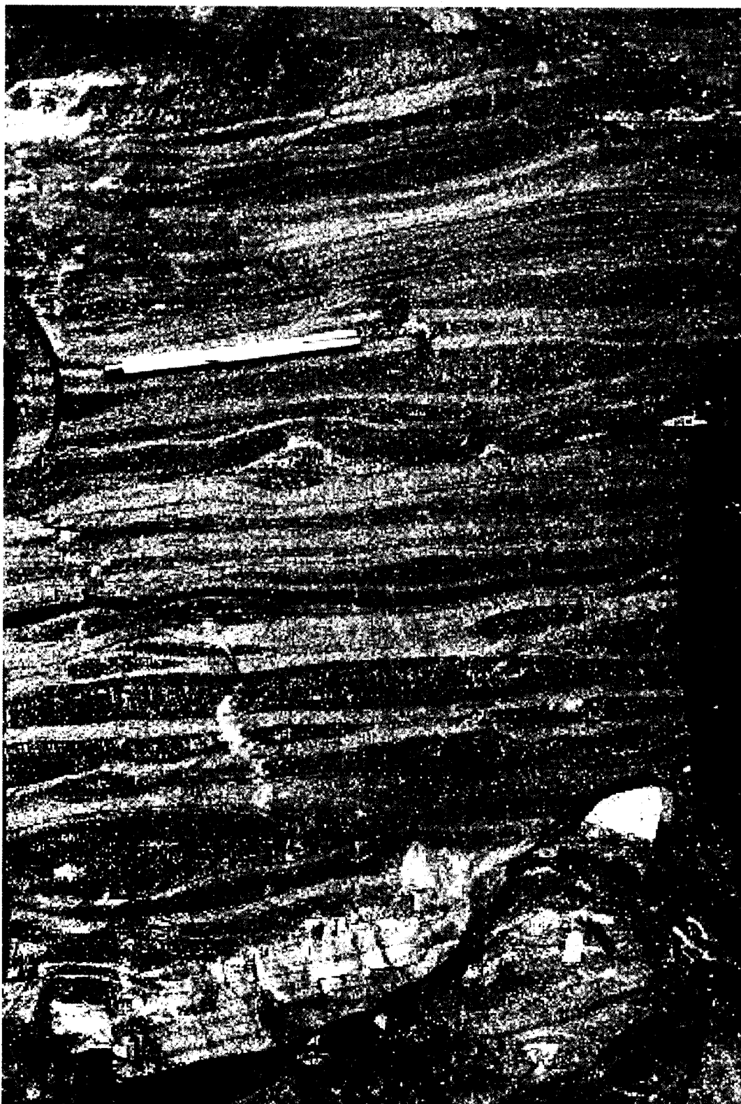
Figure 4-2. Wavy-bedded jaspilite typical of the ore zone for the Republic open pit. Lighter layers are specular hematite and darker layers are lenticular beds of metamorphosed jasper.
