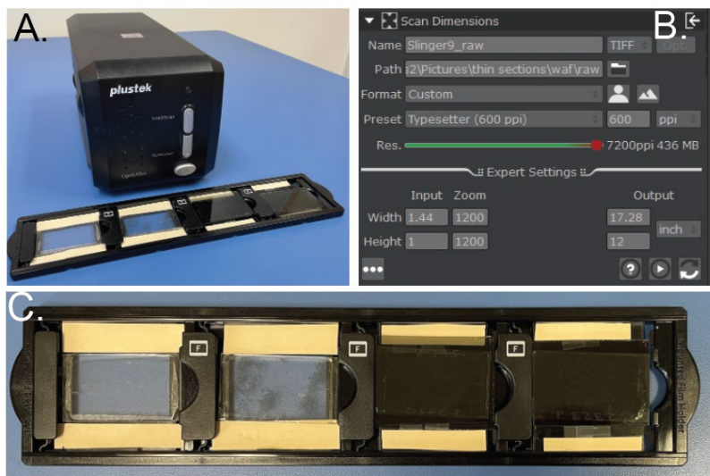
Figure 1: A) Plustek Optic Film 8200i scanner and accompanying film tray. B) Scanner settings to be used during the proposed project. Note the 600 ppi preset and further 7,200 ppi adjustable resolution. Thin sections are scanned in 48-bit HDR Raw C) Tray with card stock paper cut to better hold thin sections. Note the two slots on the right are fitted with linear polarizing screens that sandwich the thin sections. The polarized screens are oriented to cross polarize the light when scanning.
