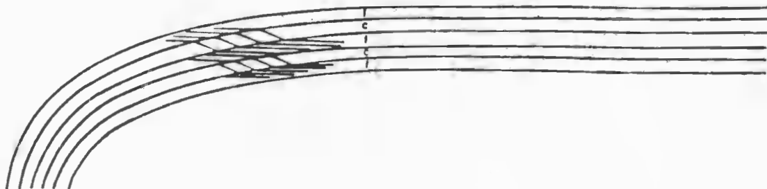
Figure 10: Position on early large-scale isoclinal recumbent fold (nappe) of cleavage refraction pattern shown in Figure 9B.
