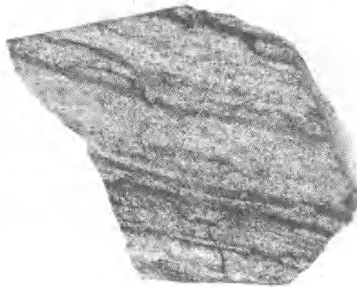
Figure 31. Hand specimen of micaceous, clay-rich quartzite from Veedum, locality 1. Dark beds are quartz-rich, lighter beds are rich in sericite partially altered to clay.
