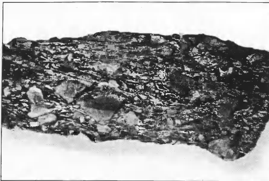
Figure 16. Photo of sawed slab of Emperor Volcanics from Stop 9. Larger, angular felsite clasts in a finer grained, foliated hyaloclastite matrix. Slab is 18 cm long.
