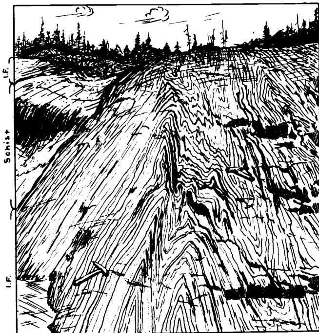
FIG. 3 (LEFT) SKETCH FROM PHOTOGRAPH SHOWING NATURE OF ISOCLINALLY FOLDED IRON FORMATION AS SHOWN IN FIGURE 2. VIEW IS LOOKING TO THE NORTHEAST IN THE DIRECTION OF THE FOLD PLUNGES.
