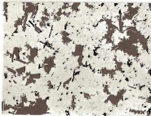
As M. 500x Hematite, white; and gangue and pores, dark grey.
