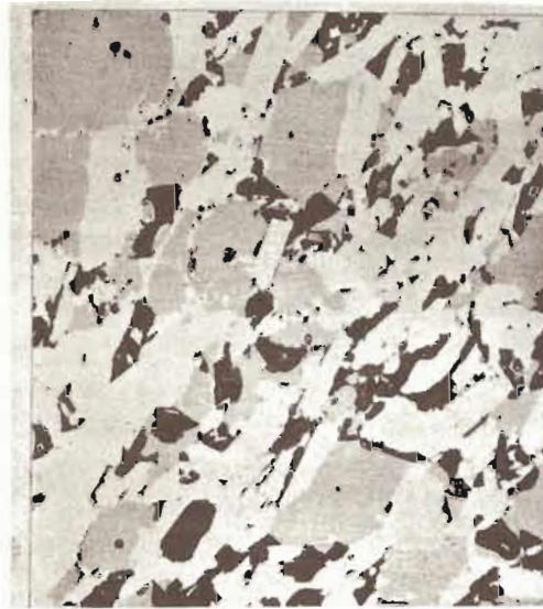
K. Specularitic Cherty I-Fm. Pol. Sec. 100X - Hematite, white; chert, black
