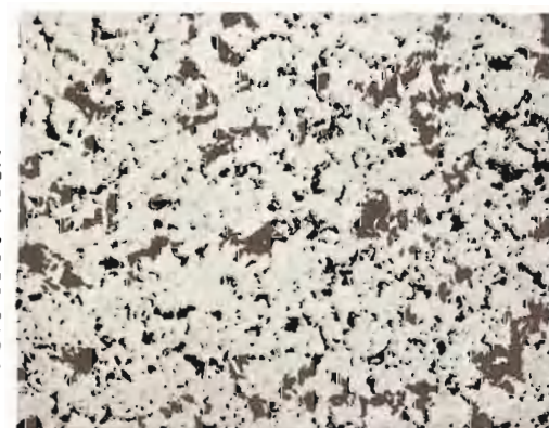
O. Mather soft martitic ore. Martite, white, chert, dark. Hematite, greyish white. Pol. sec. 100x.
