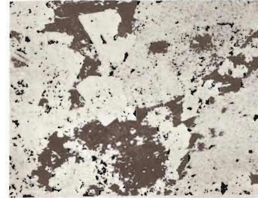
T. As S. Pol. sec. 100x Hematite, greyish white; martite, white; gangue, dark grey.
