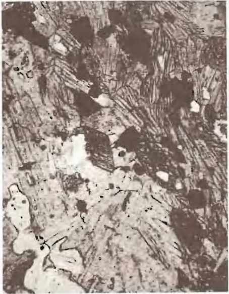
C. Mag. Grunetic Cherty I-Fm. Thin section 100X Republic Mine Grunetite, gray; chert, dusty white; magnetite, black
