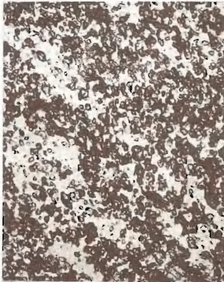
A. Cherty Carbonate I-Fm. Thin Section 200X Athens Mine Magnesium iron carbonate granules, various shades; chert, white
