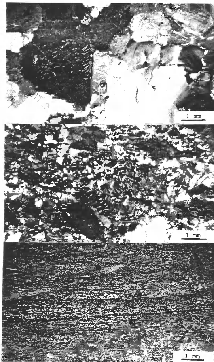
Figure 15. Photographs showing the progressive cataclastic degradation from an undeformed granite (top) to mylonite (center) to ultramylonite (bottom). The protolith for the mylonite can be established where the transition is exposed.
