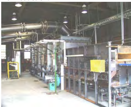
Figure 3: Pilot Scale Linear Hearth Furnace (Rotary Hearth Simulator)
