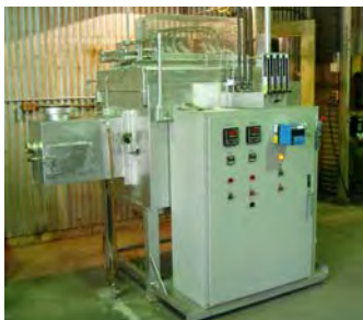
Figure 2: Laboratory Box Furnace Pilot-plant Linear Hearth Furnace Tests (Rotary Hearth Simulator)
